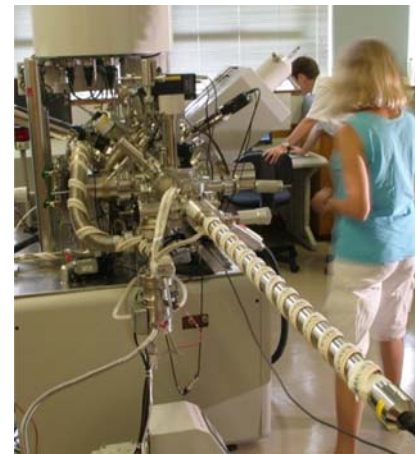
Fig. 3 The Kratos Axis DLD XPS system in the Research Centre for Surface and Materials Science at the University of Auckland
